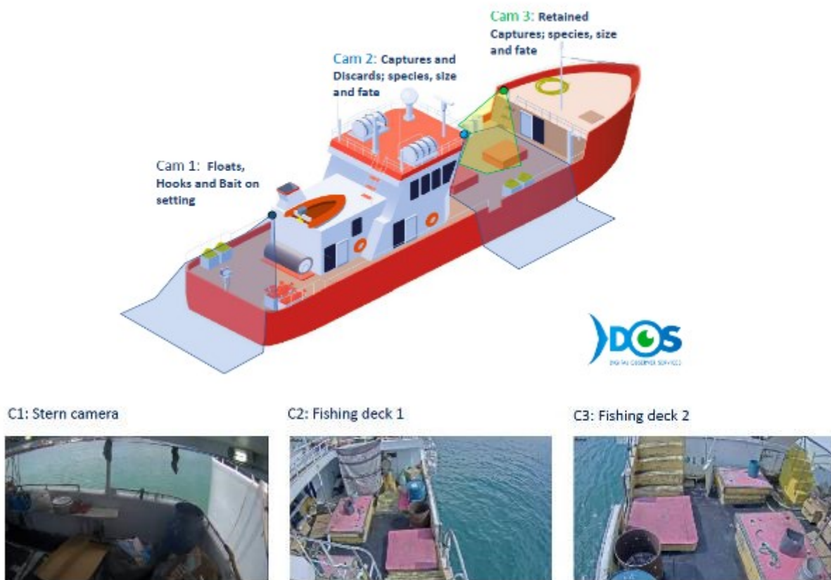
Figure 2. An example of a 3-camera EM equipment installed on a longline covering main areas of fishing and fish handling operations. View of the 3 cameras: (left panel) Stern camera - setting longline providing information on hooks, floats, mitigation techniques and bait; (middle panel) Fishing deck 1 - hauling information, captures and discards, species ID, size and fate; and (right panel) Fishing deck 2 - fate of the species, size, species ID (source: Digital Observer Services).
